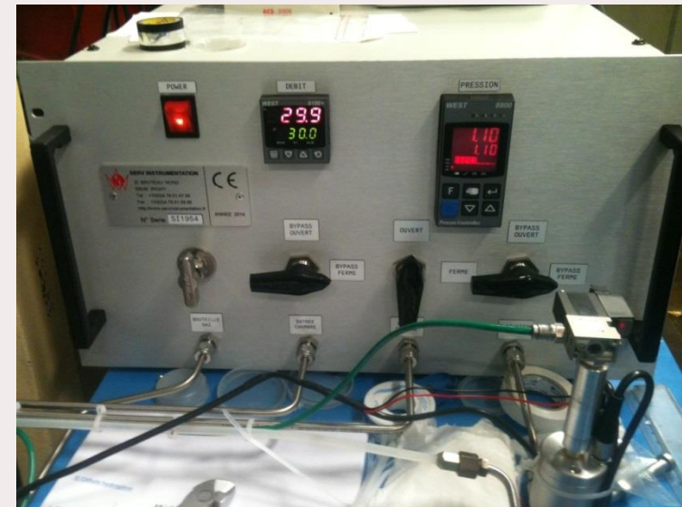
H 2 pressure and low control system
