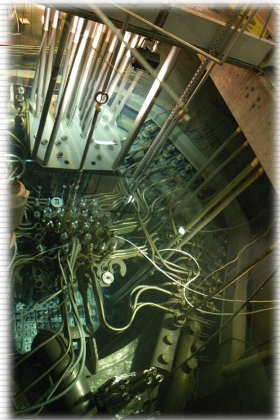
MARIA RR started with fuel conversion program according to RERTR Initiative (Reduce Enrichment for Research and Test Reactors) is in progress **19.75% / 485 g U-235 per FE / density of 4.8 g/cm<sup>3</sup>**
