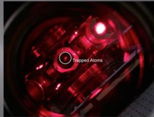
Figure 7. The source excites Ne atoms into the metastable state using an rf resonator. The red color is of the ^3P_2 - ^3D_3 neon trapping transition.
